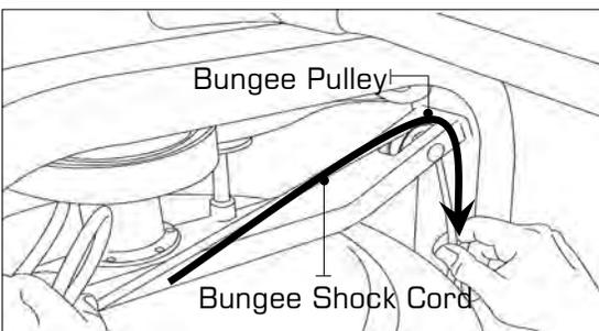
Rethread the Bungee Shock Cord (on opposite side of the Idle Wheel) back through the Bungee Pulleys and tie off at the Attachment Point.
