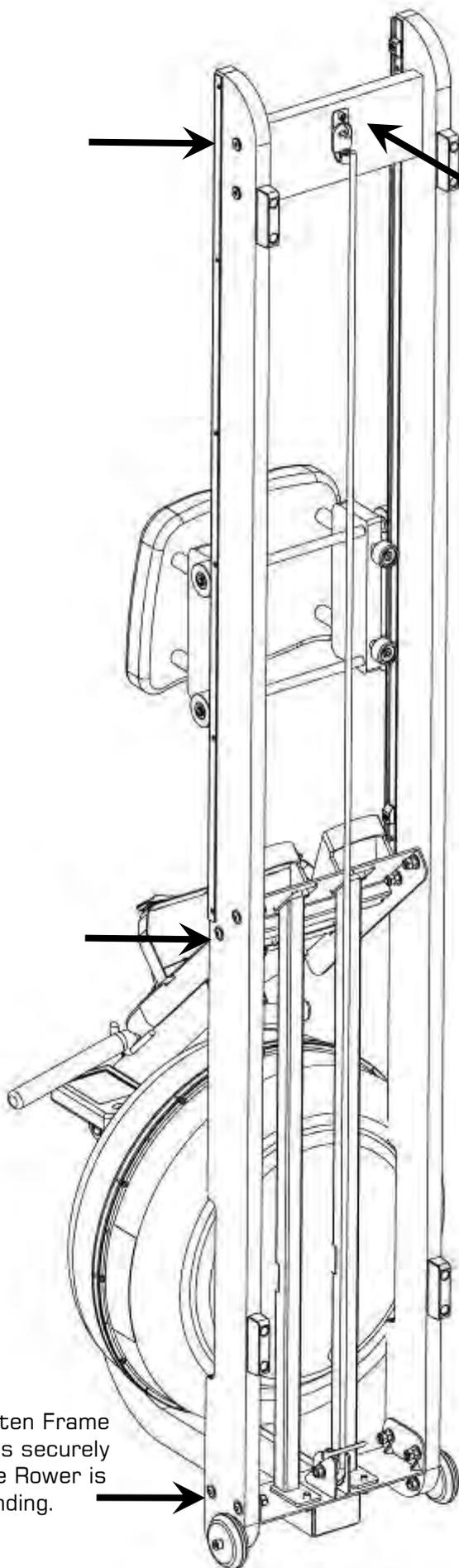
Tighten Frame Bolts securely once Rower is standing.
