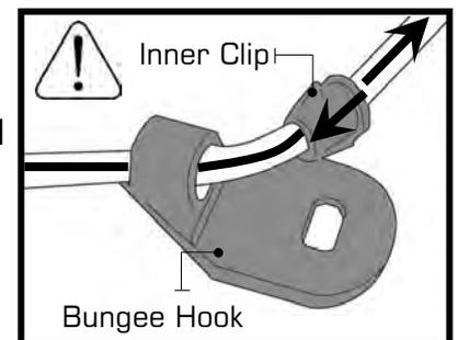
**Hint:** Before reattaching the Inner Clip/ Bungee Hook, tie a slip knot under slight tension at the lower bungee pulley. This will keep the bungee under tension while reassembling the Bungee Hook.
